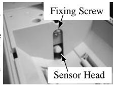
a fixing screw and a sensor head in the wall. Slightly release the fixing screw using a blade screw driver or suitable coin to adjust the position of sensor head. For smaller roll diameter, the sensor head should go lower.
