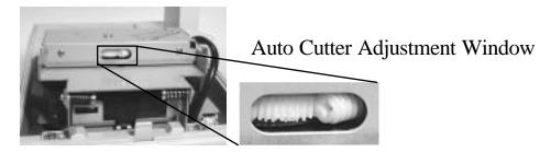
To check for home position of the auto cutter, please open the auto cutter and look into the blade slot and the spindle hole as in pictures below. Use proper tool to cut away the paper around auto cutter if it presents obstacle to the actions. Clear away any paper scraps from the auto cutter once it is reset to position.
