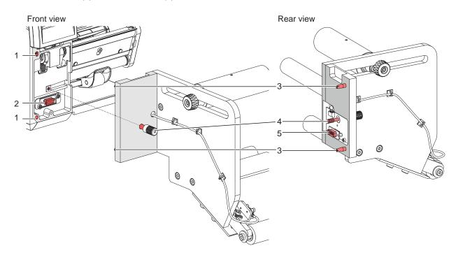
Fig. 3 Mounting the demand module
