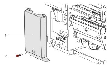
Fig. 2 Mounting the demand module
