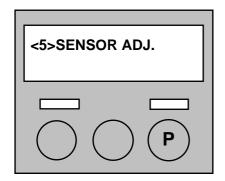
**4.** Press the **[PAUSE]** key to enter the Sensor Adjustment Mode.
