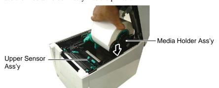
Slightly push the Upper Sensor Lever inside (①), and open the Upper Sensor Ass'y (②).
