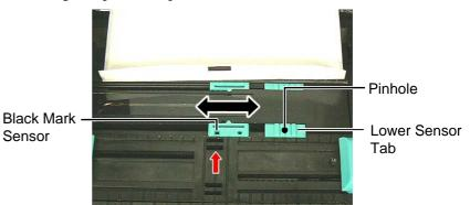
(4) Lower the Upper Sensor Ass'y until the Upper Sensor Lever clicks in position.
