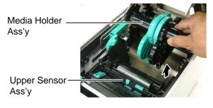
**3.** Raise the Release Lever and remove the Media Holder (Left).
