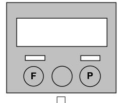
**1.** While holding down the **[FEED]** and **[PAUSE]** keys, turn on the printer.
