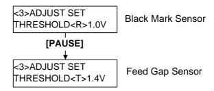
(4) Set a threshold voltage (calculated in Sensor Adjustment Menu) by using the **[FEED]** or **[RESTART]** key, as shown below.
