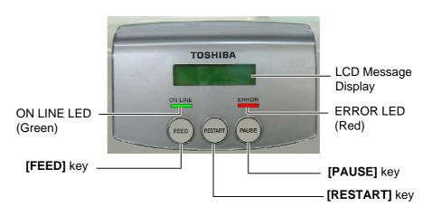
The LCD Message Display shows messages in alphanumeric characters and symbols to indicate the printer's current status. Up to 32 characters can be displayed on two lines.
