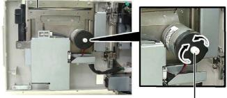
Cutter Motor Shaft \_
