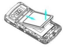
Step 1: Hold down the Power key for 5 seconds and then tap "Power off" to turn off the terminal. Slide the battery cover latch to the unlock position and remove the cover.
