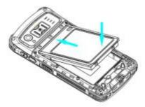
Step 1: Slide the battery cover latch to the unlock position and remove the cover.
