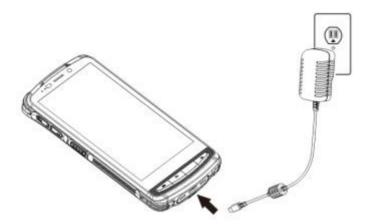
Note: Low battery may result in malfunction of the terminal. Before your first use, charge the battery for at least 8 hours.
