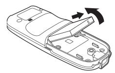
**Step 4.** Replace the back cover and secure with the Phillips head screw.
