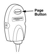
Scan the linking bar code on the top of the Access Point to establish a connection between the Access Point and the scanner. The scanner emits a short beep and flashes the green LED to confirm a connection with the Access Point. The Access Point's Page button remains blue.
