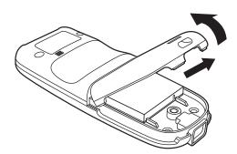
Step 3. Lift out the battery and replace, making sure the contacts on the battery line up with the contacts in the scanner.
