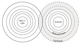
Scan one of the bar codes below to set the scanner's power output to **Full Power** (100%), **Medium Power** (35%), **Medium Low Power** (5%), or **Low Power** (1%). *Default = Full Power*.
