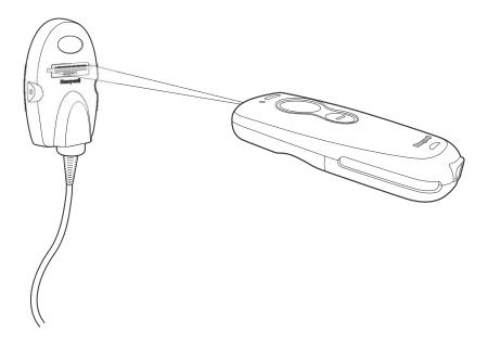
If the Access Point sounds 5 error tones followed by 3 beeps, it indicates that you are attempting to link to the incorrect model Access Point. The Voyager 1602g scanner can only link to an Access Point model AP01-010BT or AP01-100BT.
