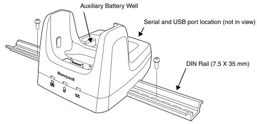
Slide the DIN rail slot along the bottom panel.
