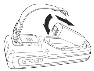
4. Replace the battery door. Apply pressure to engage the door latch.
