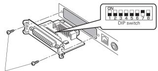
Serial interface board mounting screws
