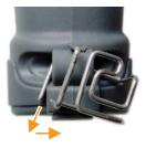
3. Attach the bottom part of the cable clip to the scanner handle.
